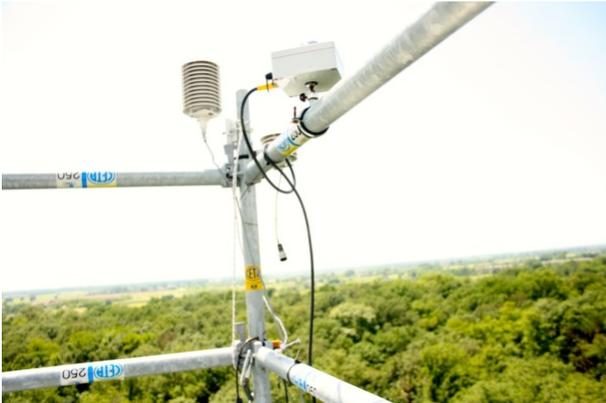
***Radiation probes on the top of the tower***
