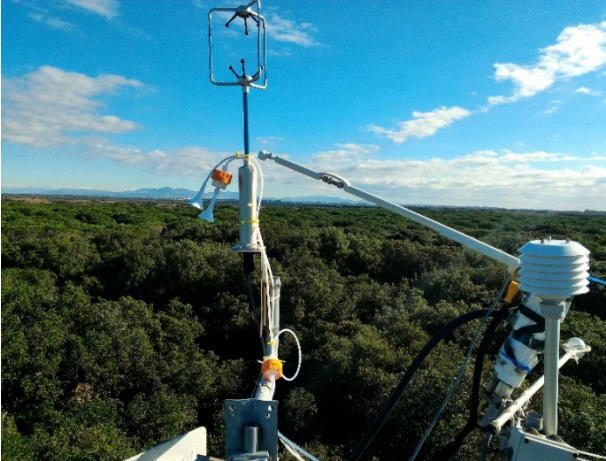
Flux monitoring system at the top of the tower
