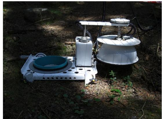
**CO<sub>2</sub>/H<sub>2</sub>O sampling system for storage flux determination**
