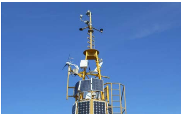
The top trellis of the buoy with the meteorological equipment.
