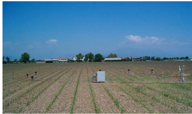
The CO 2 automatic chamber system during early corn crop development.
