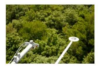
Micrometeorological instrumentation on the top of the tower
