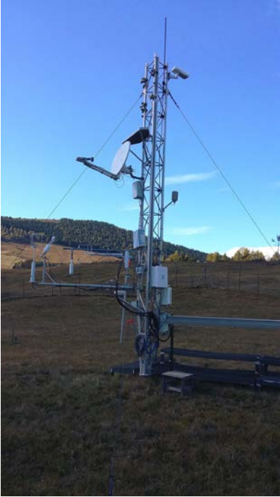
Eddy tower with typical setup Li7200 and Li7500
