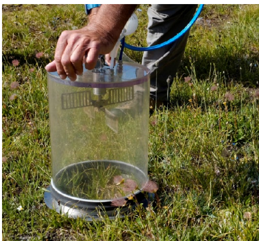
CO 2 accumulation chamber for measuring Net Ecosystem Exchange (NEE, with transparent chamber) and Ecosystem Respiration (ER, with the chamber shaded by a dark cover)
